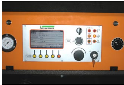
The control panel of the new arc-spray power source with all input and control elements
